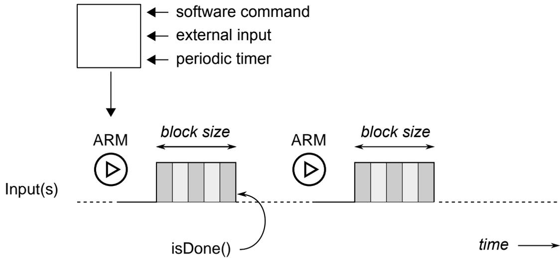
In any mode, the acquisition of timing data begins with the ARM signal. The ARM signal can be given “on-demand” by software control, external pulse, or on periodic timer intervals (Figure 2).
