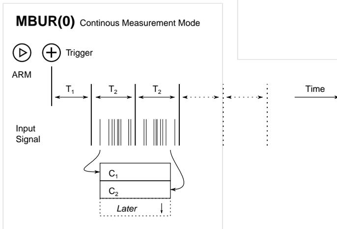
In the Continuous Mode the counter takes samples continuously after the trigger event occurred once. First, the counter waits until the trigger event occurs. After trigger, the  $T_1$  parameter specifies the delay from the trigger event until the begin of the counting window. The length of the counting window is defined by the  $T_2$  parameter.
