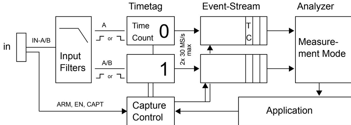
The TIC-8420 system is shown in Figure 1. After optionally low-pass filtering the inputs, the Timetag unit continuously counts edges and records the time of their appearance. At the same time, the Capture Control unit decides when to capture a count-time pair (event) into the Event-Stream.
